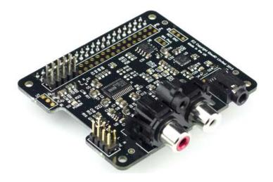
The IQaudIO Pi-DAC+ audio card for the Raspberry Pi delivers outstanding sonic performance and full-HDaudio capability with build-in hardware volume control.
